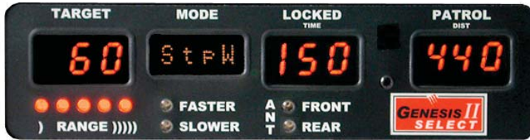
Figure 6.9 The Mode window will display "StpW" whenever the Genesis II Select™ is operating in the Stopwatch Mode
