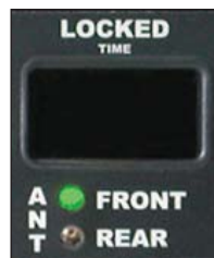
Figure 3.2.2.4b Antenna lights showing front antenna is active
